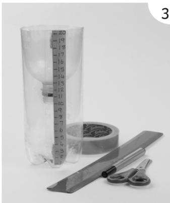
3 Make a scale in centimetres on a piece of tape, using a ruler, and fix it to the side of your bottle. You could use the Rain Gauge Scale to help you.
