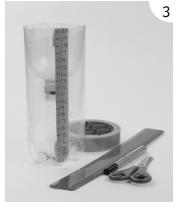
Make a scale in centimetres on a piece of tape, using a ruler, and fix it to the side of your bottle. You could use the Rain Gauge Scale to help you.
